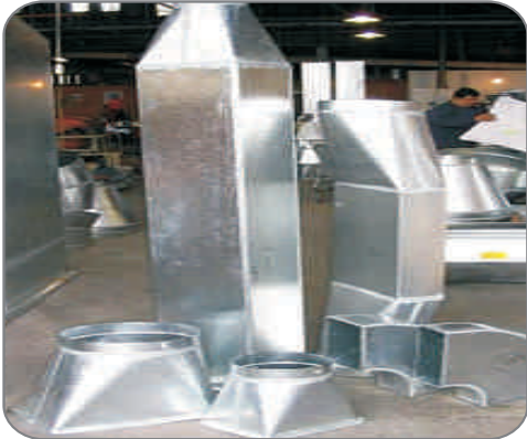
GI SQUARE DUCTING
