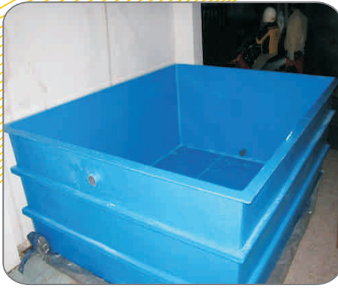
F R P WORK IN M/S TANK
